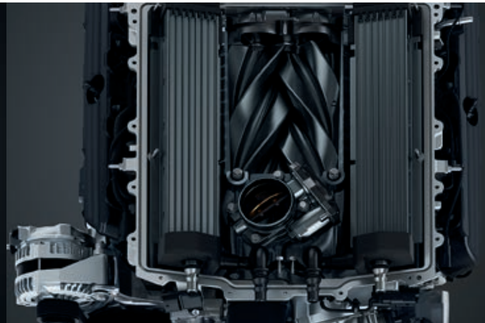
EATON SUPERCHARGER HAS 52% GREATER CAPACITY THAN ITS PREDECESSOR.
