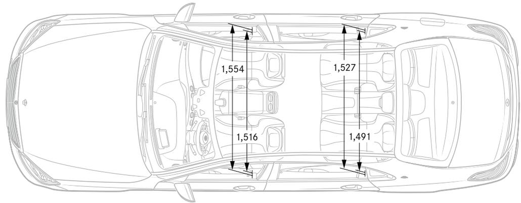
All measurements in millimetres. The dimensions shown are mean values and apply to standard-specification, unladen vehicles. Dimensions may vary slightly depending on the engine. Please consult your Retailer for further information. The figures on pages 44–45 are correct at time of publication. Please refer to the government website for latest data – <http://www.dft.gov.uk/vca>
