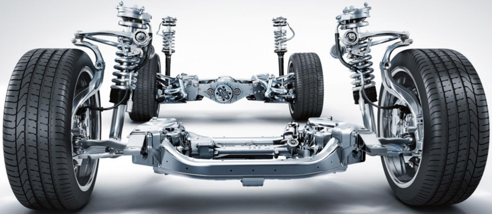
MAGIC BODY CONTROL detects bad road surfaces in advance and reacts accordingly. The active damping system of the suspension works with a road surface scan to achieve this
